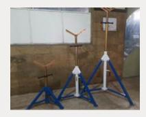
Danish Technological Institute, Certification & Inspection, hereby certifies that the welding stand with type designation Pipe stand Heavy Duty HD 2725 kg - Medium, has been subjected to an overload test with 25% overload = 3410 kg. The product was found to meet the requirements to mechanical stress as stipulated in the Machinery Directive 2006/42/EC (appendix 1, par. 4.1.2.3 b) with revisions.
