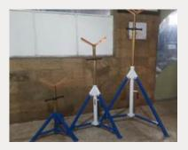
Danish Technological Institute, Certification & Inspection, hereby certifies that the welding stand with type designation Pipe stand DWT Heavy duty HD 2725 kg - Large, has been subjected to an overload test with 25% overload = 3410 kg. The product was found to meet the requirements to mechanical stress as stipulated in the Machinery Directive 2006/42/EC (appendix 1, par. 4.1.2.3 b) with revisions.
