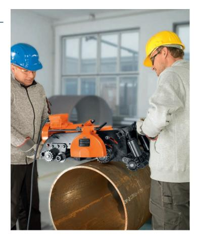
Safe use: The feed motion can be switched on and off and the integrated safety slip clutch protects the feed gear from overload.
